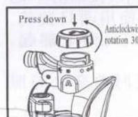
Press to rotate 30° anticlockwise to open battery compartment
